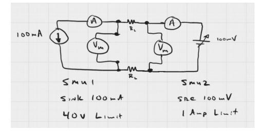
SMU1 measures only 61mV. The remaining 39mV is dropped across the two  $R_L$ .
